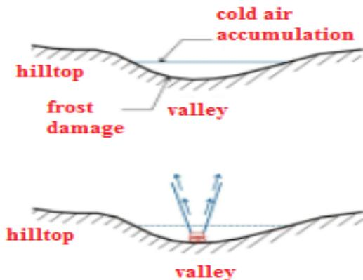
**Figure 1.** Selective Cold Air Drainage
