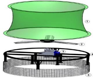
**Figure 5.** Parts of upward-blowing wind machine are; 1. Fan Chimney, 2. Fan Kit, 3. Engine, 4. Construction 5. Protection cage.
