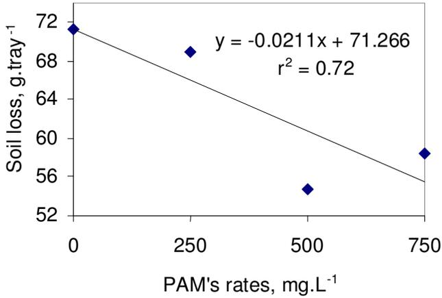
Figure 7. Relationship between soil loss and PAM application rates.
