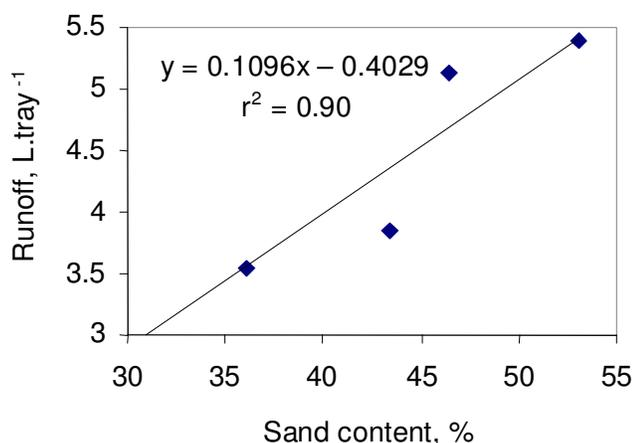
**Figure 13.** Relationship between runoff and soil sand content.
