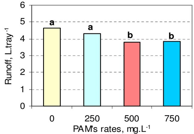
Figure 10. Runoff for different application rates of PAM. Columns labeled by the same letter do not differ significantly at the 0.05 level.
