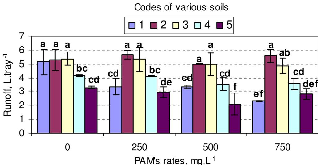
**Figure 12.** The interaction between the different application rates of PAM and various soil types in terms of the effects on runoff.
