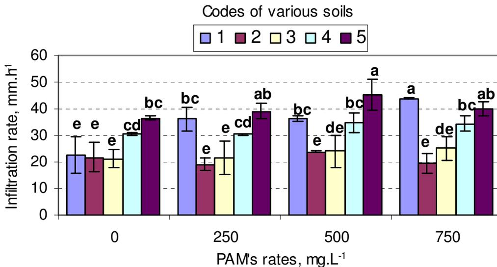
**Figure 18.** The interaction between the different application rates of PAM and various soil types in terms of the effects on infiltration rate.
