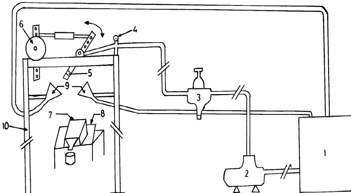
Figure 2. Schematic structure of the rainfall simulator and its parts ((1) water reservoir; (2) pump; (3) regulator; (4) pressure gauge; (5) nozzle; (6) electric motor and variator; (7) erosion tray; (8) sloped table; (9) excess water collectors; (10) main frame).
