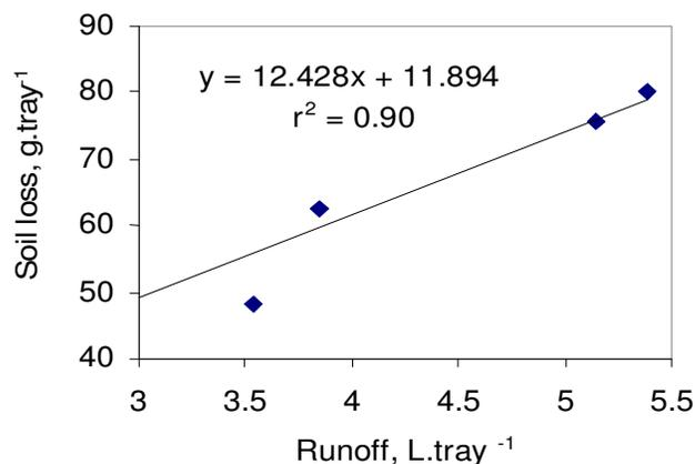
**Figure 14.** Relationship between soil loss and runoff.
