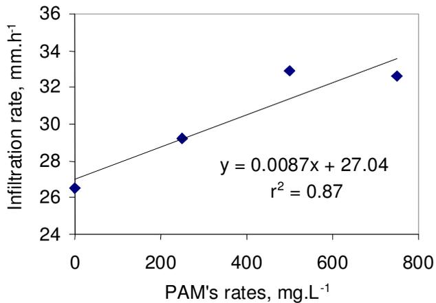
**Figure 16.** Relationship between infiltration rate and PAM's application rates.
