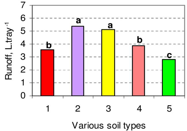
Figure 9. Runoff water from various soil types after PAM applications. Columns labeled by the same letter do not differ significantly at the 0.05 probability level.
