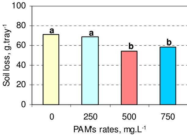
Figure 8. Soil loss for different application rate of PAM. Columns labeled by the same letter do not differ significantly at the 0.05 probability level.
