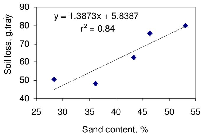
**Figure 4.** Relationship between soil loss and sand content.
