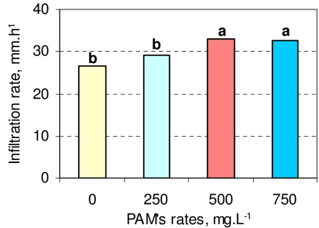
**Figure 17.** Infiltration rate for different application rates of PAM. Columns labeled by the same letter do not differ significantly at the 0.05 probability level.
