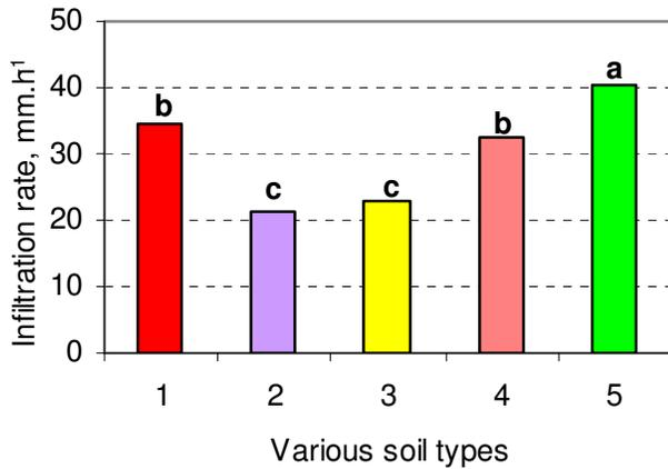
**Figure 15.** Infiltration rate from various soil types as a function of PAM's applications. Columns labeled by the same letter do not differ significantly at the 0.05 probability level.
