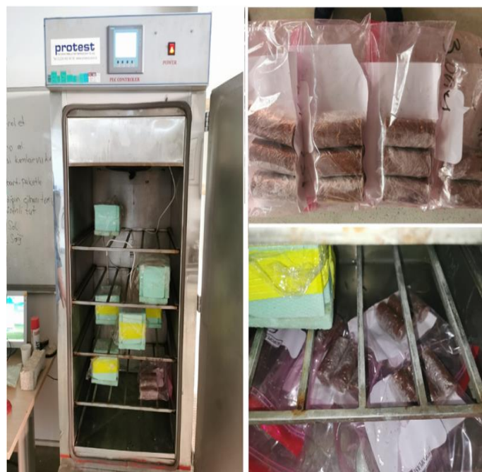
Figure 3.11. Soil specimens' preparation in the freeze-thaw cabinet before triaxial testing.
