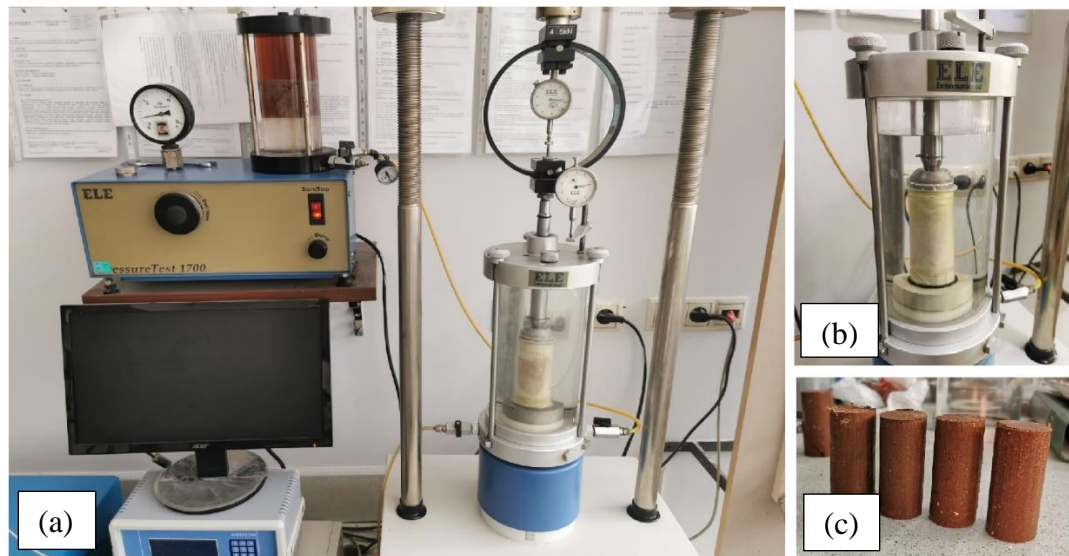
Figure 3.6. Undrained unconsolidated triaxial testing: (a) Unconfined unconsolidated triaxial machine used, (b) Specimen preparation for testing, (c) Specimens before testing.
